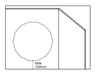
Sensor needs to be a minimum 150 mm away for any surface
